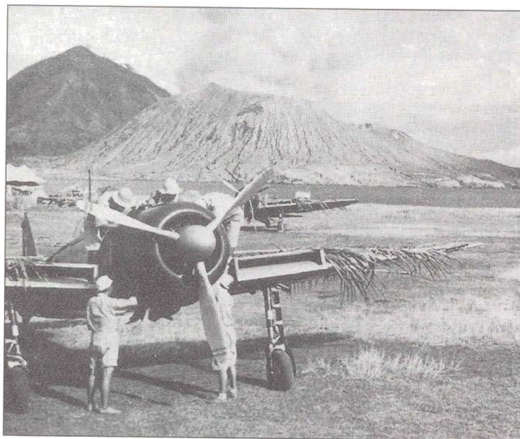
Mechanics labour over a Zero 21 at Lakunai airfield as Mt Hanabuki belches smoke in the background – the active volcano being a familiar landmark for pilots approaching Rabaul. Field modifications performed on the Zero included sawing off the radio mast and removing the useless radio to in order to save weight
